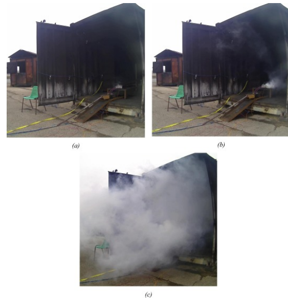
Figure 4. Mechanical abuse of a lithium-ion battery module at 50% state of charge (SOC). The gas cloud produced contained HF, CO 2 , CO, H 2 , e HCN [2]. Reproduced with permission from [2].
