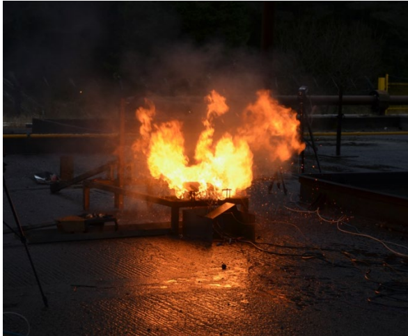
Figure 1. Fire propagation in a module made up of 8 (lithium nickel manganese cobalt pouch cells) in a thermal abuse experiment in 2019. Picture taken by the author.
